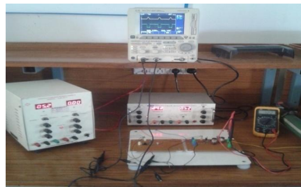
Fig. 13. Experimental set up of ZVS buck converter on work bench
